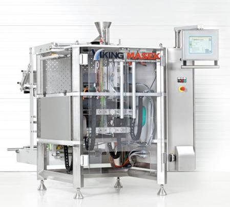
Patented, independently phased, twin sealing jaws separate the Velocity from all other high speed machines, and virtually eliminate lost cycle time. This is the fastest VFFS machine in the world – no competition.
